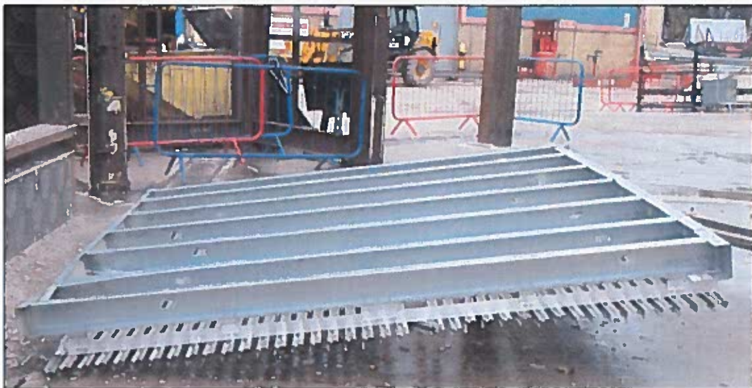
SUPPORT FRAME REMOVED FROM TEST RIG
