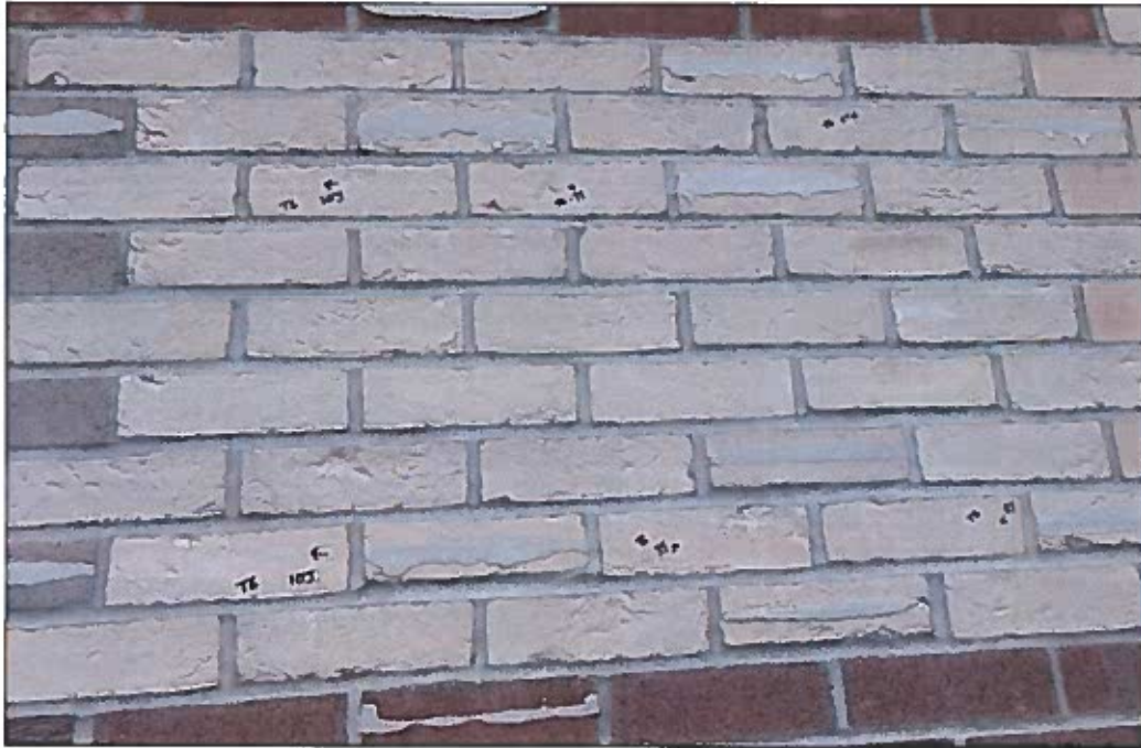
BRICK TYPE 6 AFTER IMPACT TESTS
